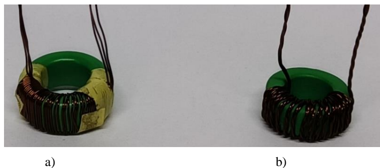
Fig. 8: a) PT3: Conductors of three windings are wound one after the other (see Fig. 7a), and, c) The proposed PT4: 3-conductor litz-wire wound as a single winding (see Fig. 7b).
