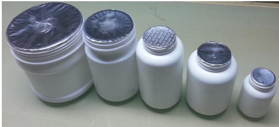
Fig. 1: Sealed containers using induction heating principle.
