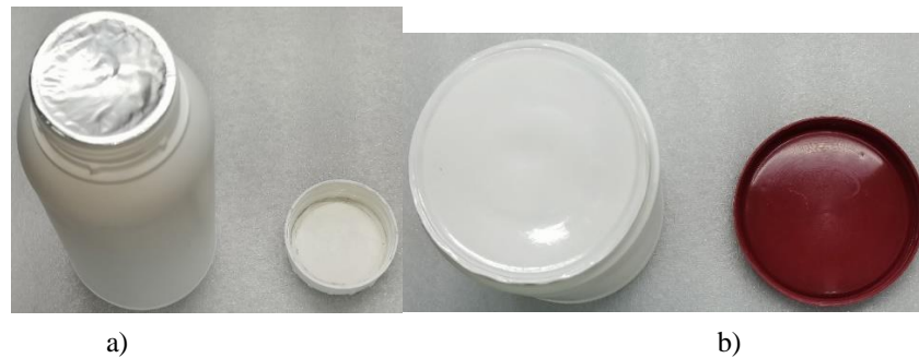
Fig. 13: Sealed containers, a) foil diameter: 55 mm, and b) foil diameter: 95 mm.
