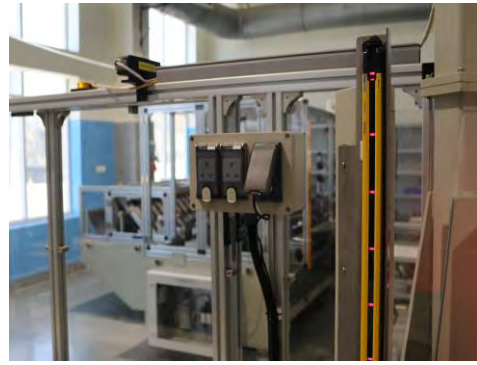
Picture 8 Hazard 1.5, Image 2, Safety magnetic door switch
